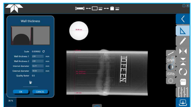
Wall thickness measurement
