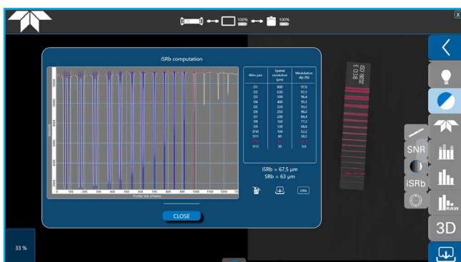
iSRb calculation and automatic IQI recognition
