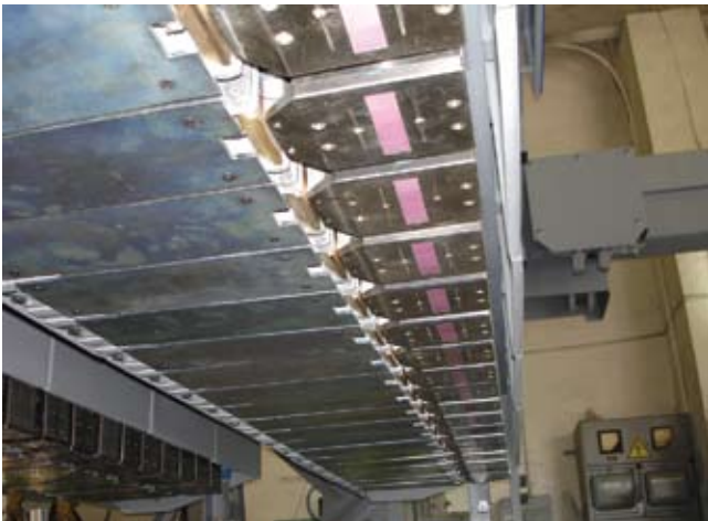
Fig. 13. Test unit of EMATEST-PL. EMATs with individual magnets – Ural Steel, Novotroitsk (Russia).
